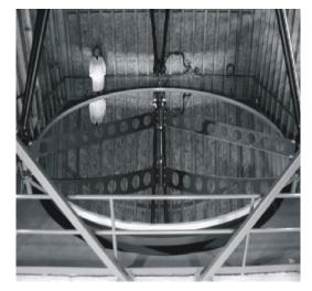
Fig. 1. The Large Zenith Telescope in British Columbia has a 6meter primary liquid mirror (Photo: Courtesy of Dr. Paul Hickson)
